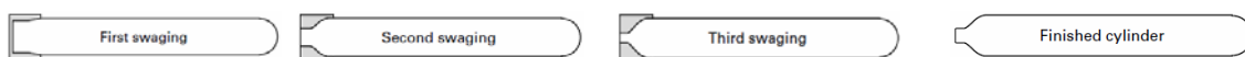
Figure 36: Steps followed in hot-swaging a tube to form the end (neck) of a pressurized gas cylinder
