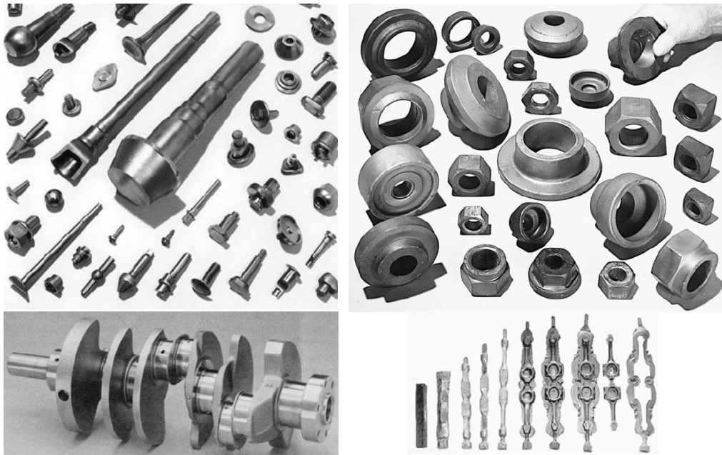
Figure 1: Typical products made by forging, rods, hubs, valve seats, fasteners, crank shaft, and connecting rod.
