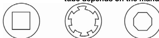
Figure 35 (c): Examples of cross-sections of tubes produced by swaging on shaped mandrels
