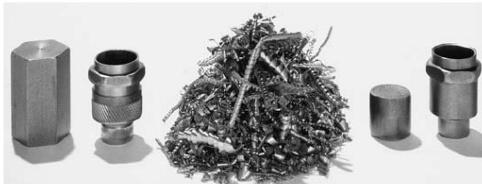
74% waste in machining Chips obtained after machining Cold forged on 6% waste Figure 5: Comparison of manufacturing of a spark plug body by machining from hexagonal bar stock with manufacture by cold forming. Material is saved, machining time and cost are reduced, and the product is stronger, due to cold work, and tougher
